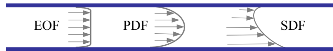
Figure 2.6 Flow profiles: simple flow profile: EOF (Electro-Osmotic Flow), PDF (Pressure-Driven Flow) and SDF (Shear-Driven Flow).
