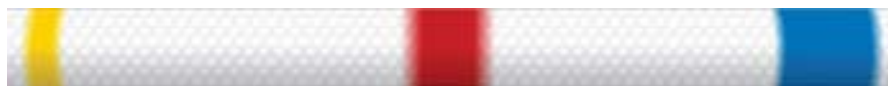
Figure 10.3 A schematic of a chromatographic column of packed microdroplets used for the separation of different components (blue, red and yellow).
